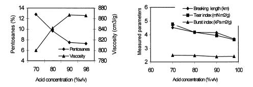
Fig. 2. Influence of acid concentration on pulp mechanical and chemical properties (cooking conditions: temperature, 100°C; time, 60 min).
