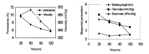
Fig. 4. Effect of cooking time on pulp chemical and mechanical properties (cooking conditions: temperature, 100°C; acid concentration, 90%).
