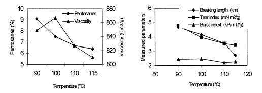
Fig. 5. Effect of cooking temperature on pulp chemical and mechanical properties (cooking conditions: acid concentration, 90%; time, 60 min).
