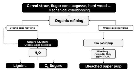
Figure 1. The CIMV process biorefinery.
