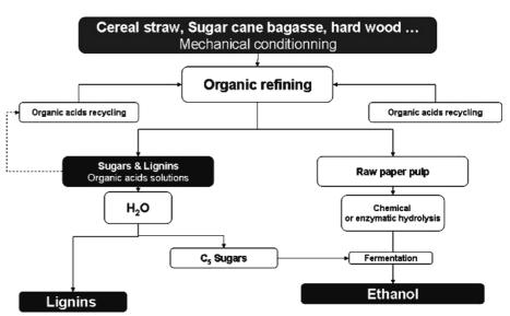
Figure 4. The CIMV bioethanol/lignins biorefinery.
